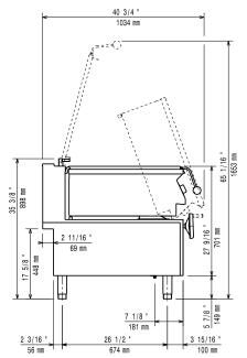
CWII Cold Water inlet 1 (cleaning) ΕI Electrical inlet (power) G Gas connection
